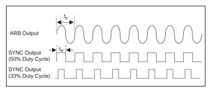
Figure 1-3. SYNC Output and Duty Cycle
